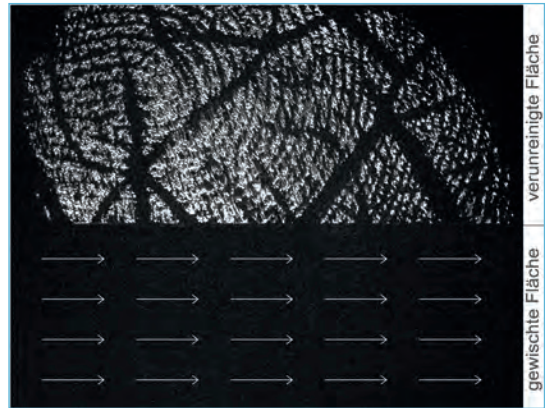
Fig. 20 Cleaning of the lower print with N-hexane and decontaminated cleaning wiper, mesh density 1056. The surface is pure.
