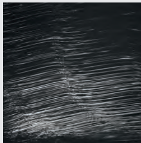
Fig. 22 Wiping of a fingerprint with non-decontaminated cleaning wiper, mesh density 400 = no residues
