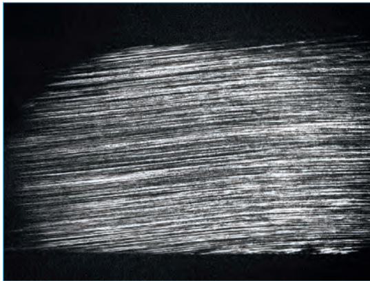
Fig. 19 Cleaning of a fingerprint with a dry polyester wiper of mesh density 300. Distinct streaks remain.
